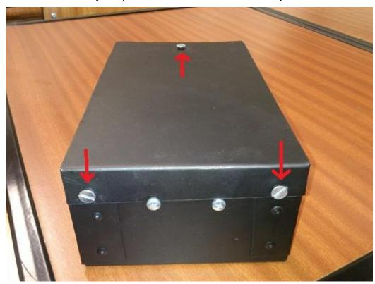
To remove the battery, it is possible to just remove it out of the box and only after remove the battery cables, this has to be done carefully not to harm the control system just next to it.
