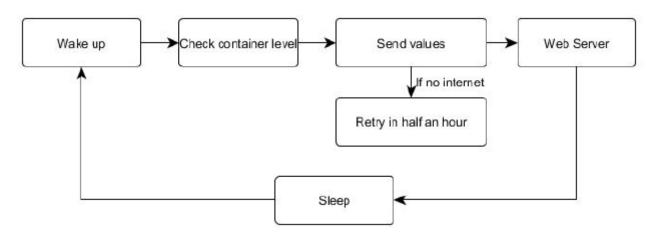
This diagram shows the basic system function, after the system checks the container level the data is processed and sent via wifly after this all the values are reseted inside the microcontroller but in the web server this values are saved in a text file for later use.
