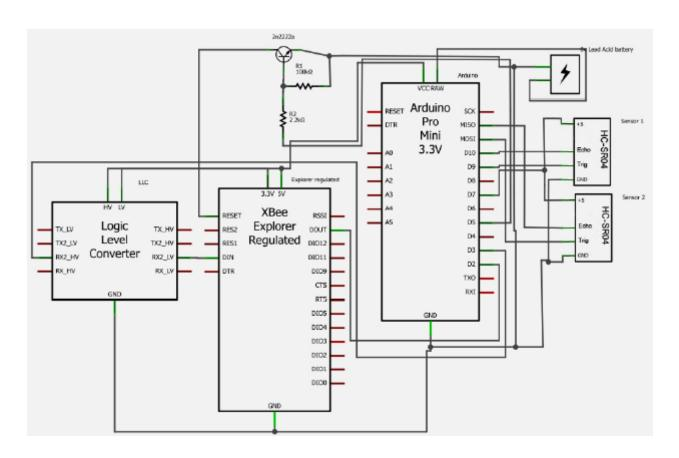
The ultrasonic sensors installed on our system provide 2 cm to 400 cm non-contact measurement function, the ranging accuracy can reach up to 3 mm. The modules include ultrasonic transmitters, receivers and a control circuit. The IO trigger is set for at least 10 us high-level signal and the Module automatically sends eight 40 kHz ultrasonic waves and detects whether there is a pulse signal back.
