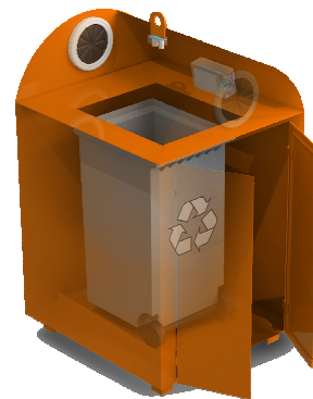
Figure 9 – Container with the level monitoring system.
